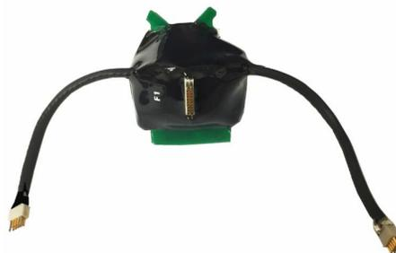
Our standard I/O connector to interface to recording electrode
