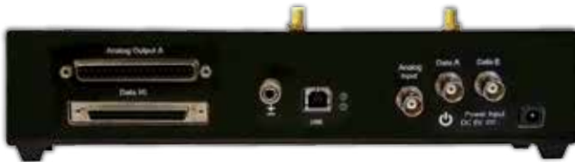
Demultiplexer Base Station Back View
