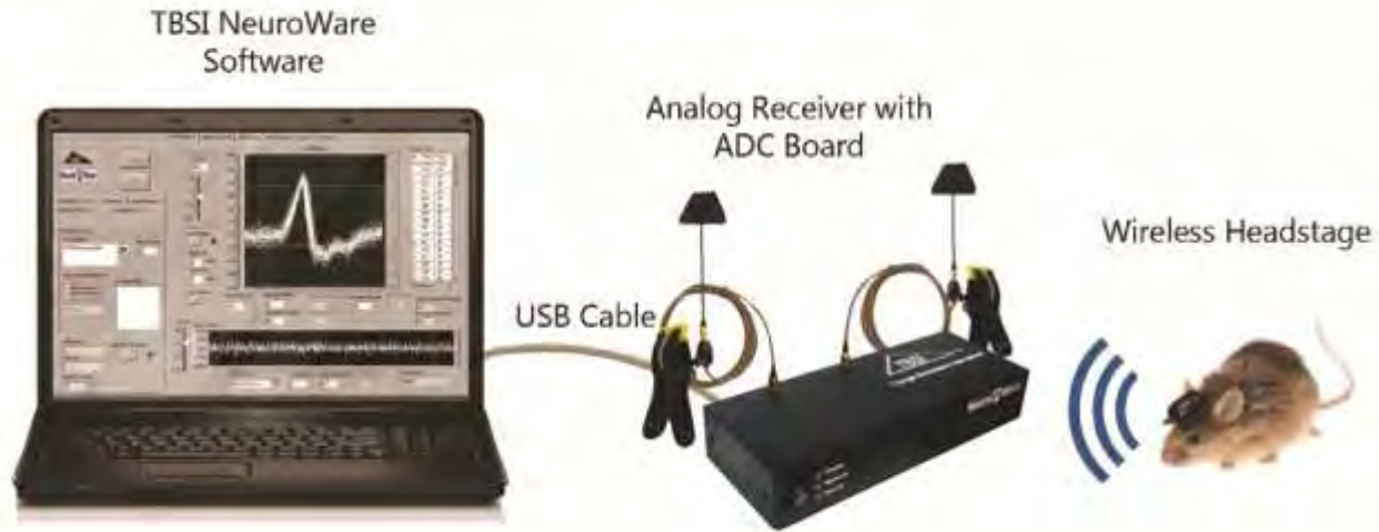
Standard TBSI Wireless Recording Setup
