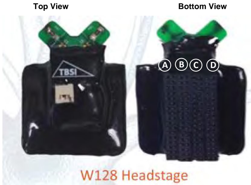
Complete headstage weight is 8.9 grams
